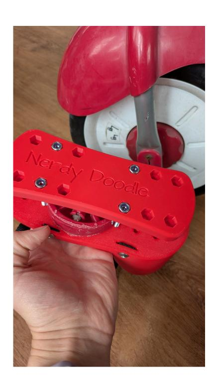
5. Place the top piece back over the pedal aligned with your bolt palcement.
