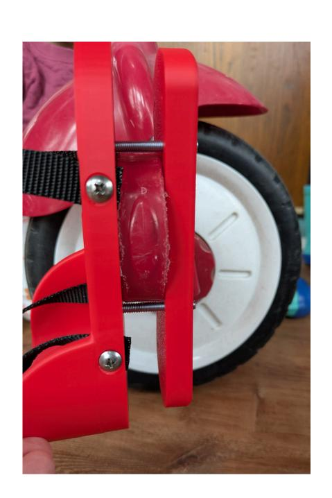
9. Use one hand to hold the adapter together and other hand to tighten bolts and secure top and bottom together.
