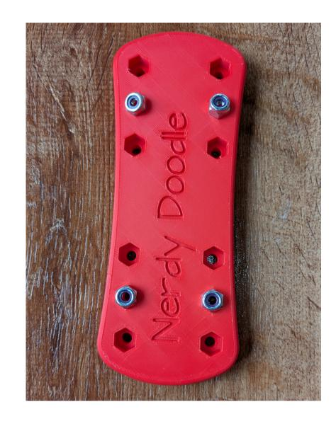
1. Place bolts through top adapter piece, determining appropriate bolt palcement based on pedal size and shape. Optimal placement is for the ball of the foot over the pedal.
