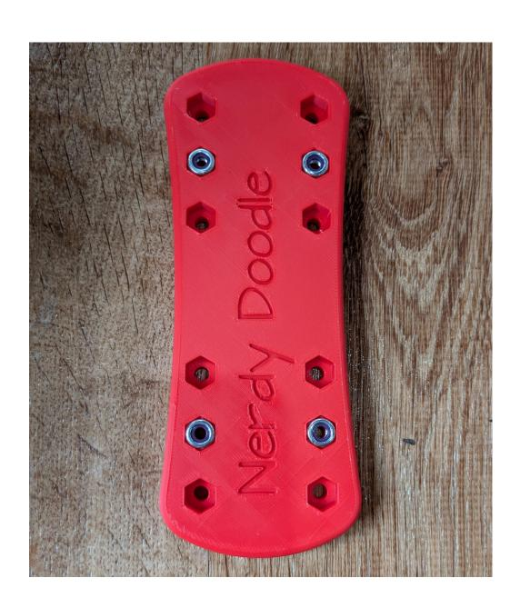
3. The locking nuts are press fit, they are a tight fit. Start pressing them in from the top, then carefully flip piece over and push firmly to slide the nuts all the way in.
